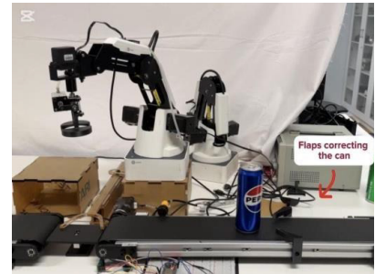
Fig 1: The can position is corrected by the flaps when placed on the belt to be in the center position of the belt.
