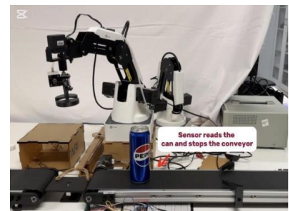
Fig 2: The infra Red (IR) sensor on the sides of the belt detects the can and stops the belt.
