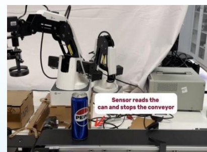
Fig 4: The can is weighed using a weight sensor underneath the platform.
